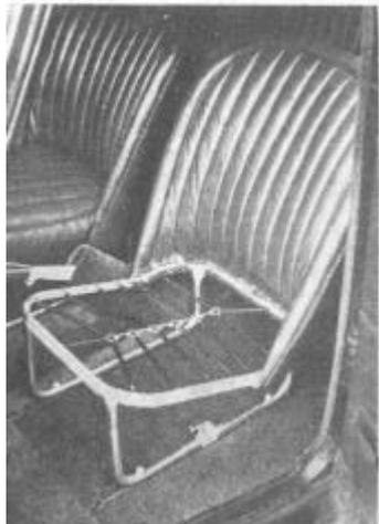
Front bucket seats were built on tubular steel frames. They are well sprung and comfortable.
