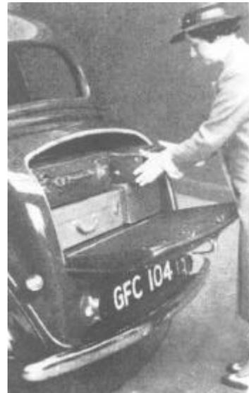
Luggage space, in the enclosed locker, is generous, the compartment being very convenient in use. Space wheel and tools are housed in a lower compartment, which is covered by the number plate.
